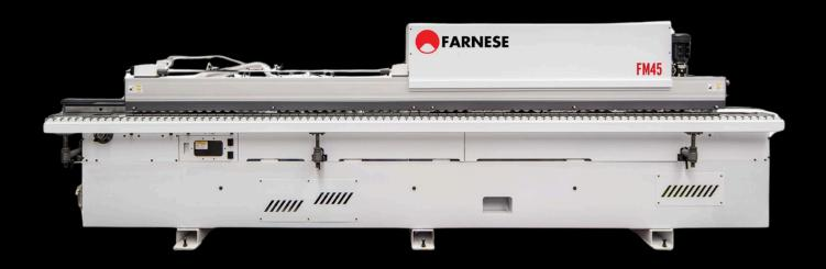
The Farnese FM45 Edgebander is a compact and sturdy machine ideal for industrial or artisan use. It features a quick-heating glue pot for efficient application of PVC and veneer edges, and it can create doors and drawers in-house with bevel, finger pull, and shark nose profiles. The units are adjusted automatically with a pressure bar provided with a double row of wheels.
