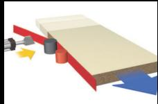
Heavy Duty Rough Trim Unit Fravol Patent Special Profile Cutters: Bevel 30, R1-3mm, flat
