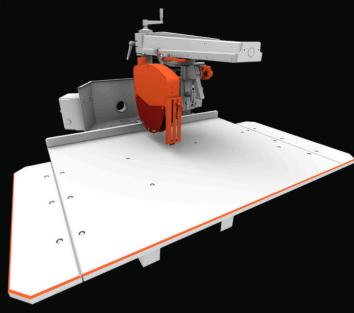
The RADIAL ARM SAWS JUNIOR 640 by Maggi Technology is a versatile and precise cutting machine designed for woodworking tasks1. It features a manual radial-arm design, allowing for straight (90°) crosscuts, miter cuts (45° left and right), and bevel cuts (45° left and right)2. This saw is ideal for furniture manufacturing and joinery, offering a small footprint suitable for small workshops.
