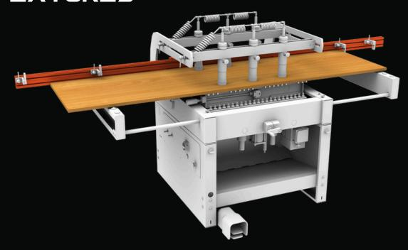
The BORING SYSTEM 46 by Maggi Technology is a semi-automatic, multispindle boring machine designed for high productivity in woodworking. It features two parallel vertical boring heads, each with 23 spindles, allowing for vertical double-row line drilling on furniture sides. This system is ideal for bookcase, bookshelf, and wardrobe manufacturers.
