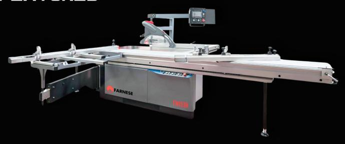
The Farnese Masterwood Australia saw machine boasts advanced features such as motorized adjustments for the main and scoring saws, electrical tilting, and a cam seat. It supports a maximum saw blade of 400mm and a cutting height of 125mm, with double scoring saw blades for precision. The table structure, processed with German technology, includes a maintenance-free sliding table and a high-precision, wear-resistant multi-cavity structure.
